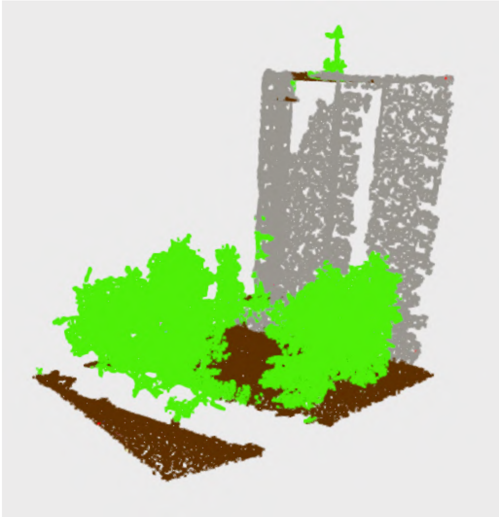
Figure 3.11: Segmentation Results with KpConv upscaled to 100 points/m 2
