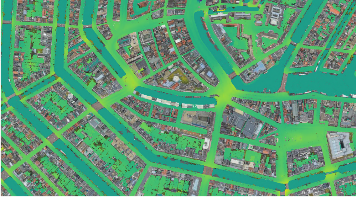
Figure 3.4: New DTM after running the River Mask algorithm
