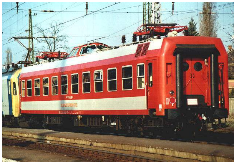
Figure 2.5: Catenary diagnostic wagon of the Hungarian State Railways 8
