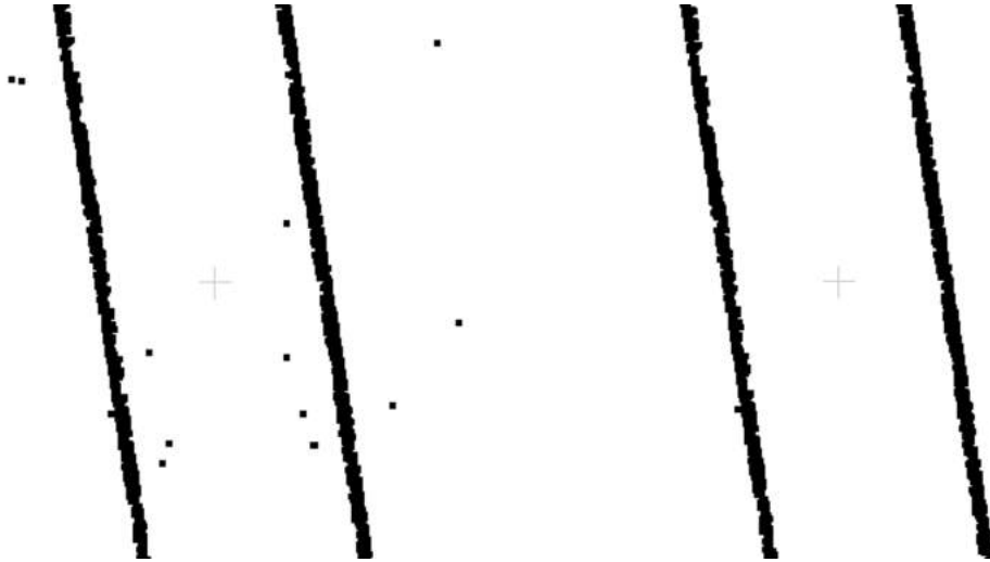
Figure 6.8: Point cloud before and after outlier-based filtering
