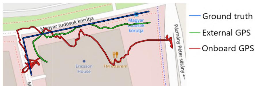
Figure 3.8: Comparison of the external GPS and onboard GNSS sensor to the ground truth
