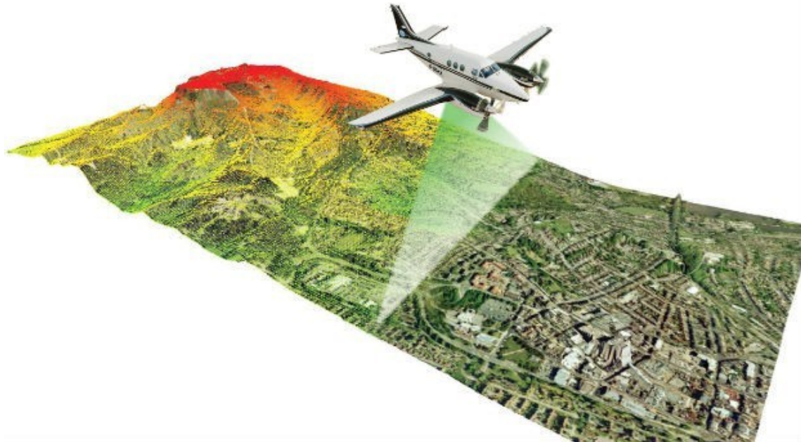
Figure 2.3: Airborne LiDAR scanning
