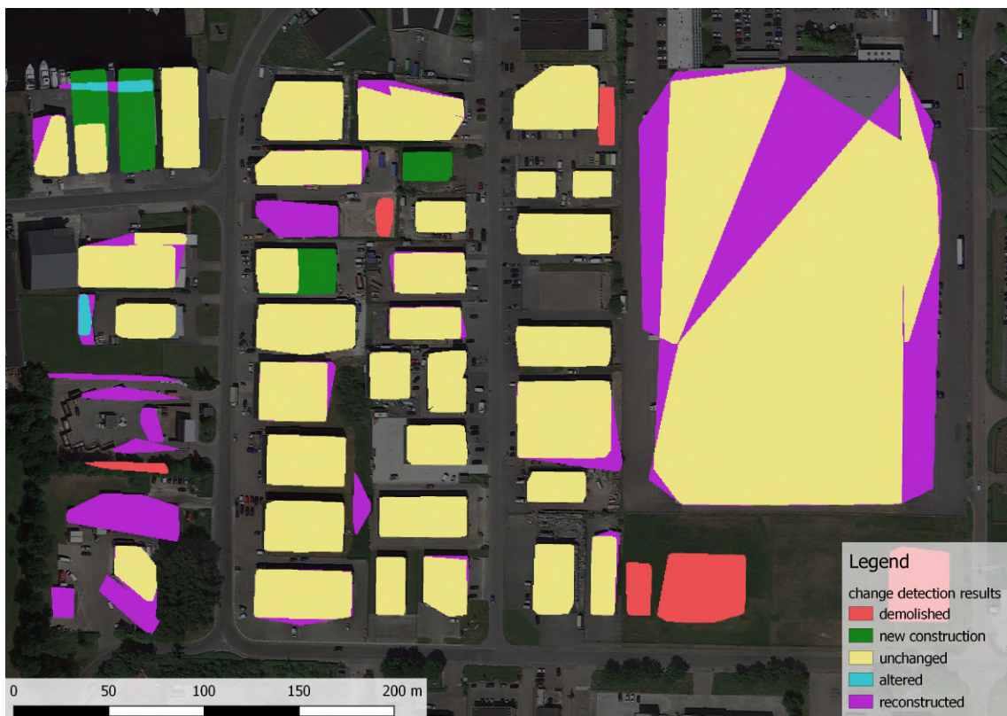
Figure 3.10: The classification result of the building change detection.
